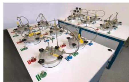
Pressurizing Helium Chamber
