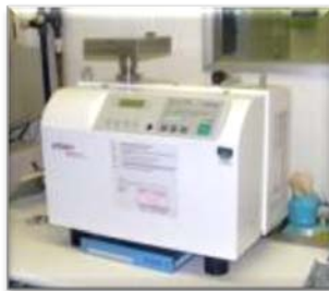
Fine Leak Test
